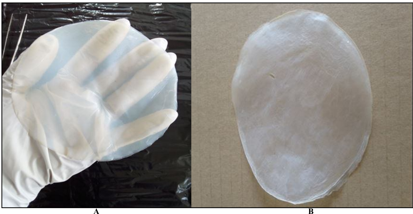
Fig. 1: A the wet thickness and B dried thickness of bacterial cellulose films.
